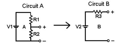
The questions ask you to find V2 and R3. To determine the equivalent single voltage source V2 in circuit B we calculate the open circuit voltage of circuit A using Ohms Law:
